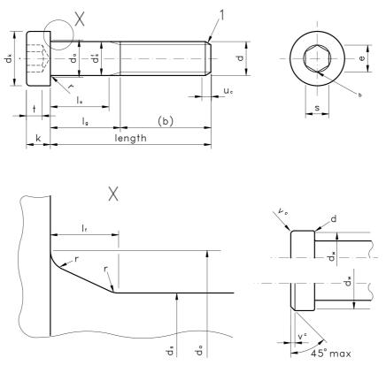
Maximum underhead fillet,  $I_{f,max} = 1.7 r_{max}$
