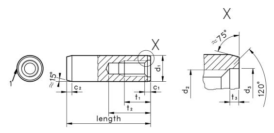
1. Slight flat or small groove at the manufacturer's discretion
