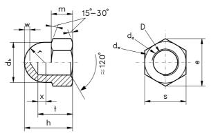
The useful thread length is given by t (thread height). x (thread run-out).
