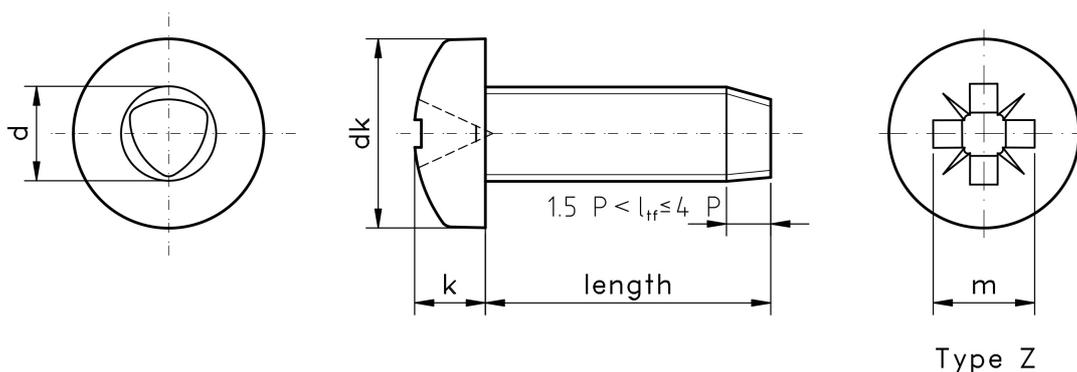
Figure 1: Pozi Pan Thread Rolling Screw
